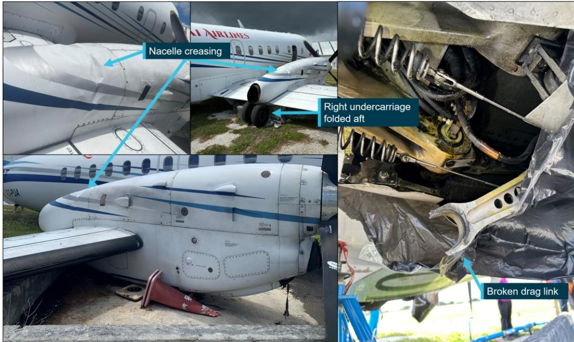
Figure 8: Right landing gear damage and broken drag link
