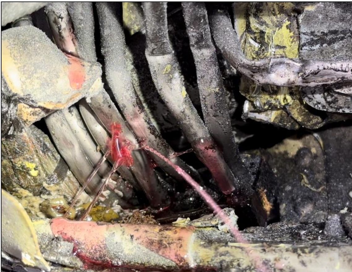
Figure 10: Crushed, cracked, and leaking hydraulic pipes
