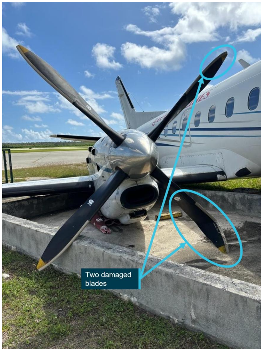
Figure 9: Right propeller blade damage
